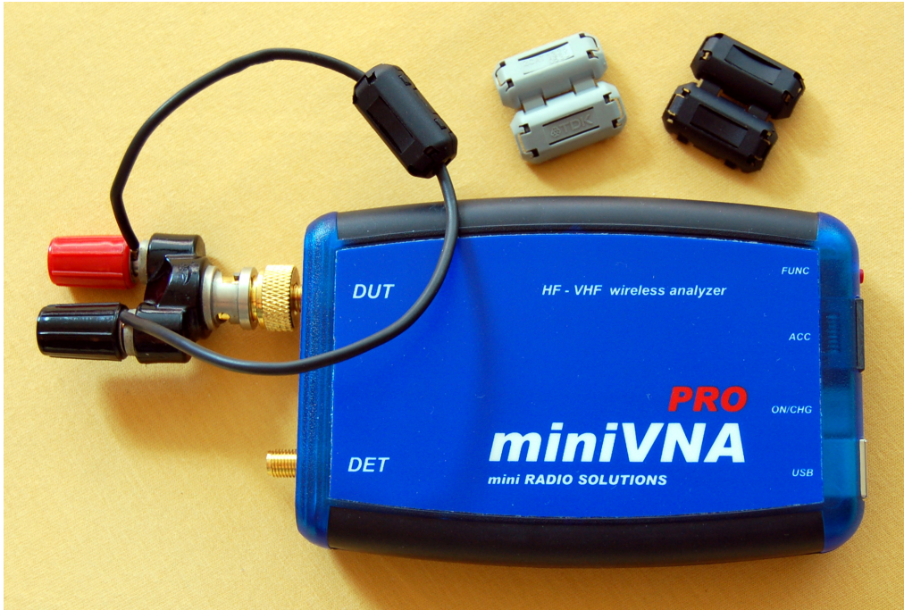
Figure 6: Choke testing with the miniVNA Pro over a wireless Bluetooth connection. The grey ferrite clamp is a TDK ZCAT 1325-0530A, the black ones are no-name counterfeit (see text).
