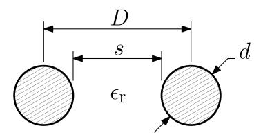
Figure 1: Parallel circular conductor transmission line; dimensions.
