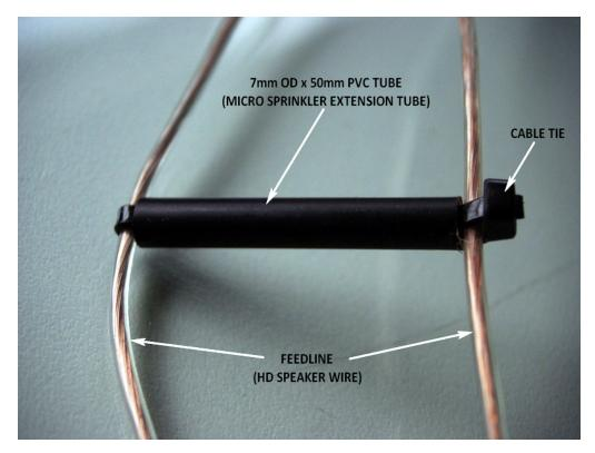
Figure 2: Ladder line spreader built from black irrigation extension tube and a cable tie. Source: Leon Salden, VK3VGA
