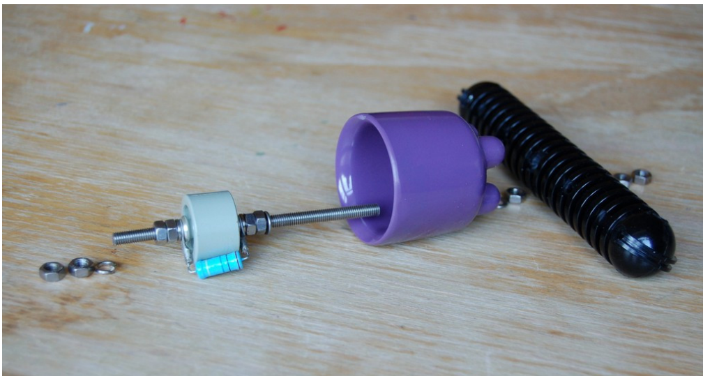
Figure 28: Layout for mounting a doorknob capacitor with its snubber resistor to an antenna insulator. All hardware is A2 stainless steel with an M5 thread.
