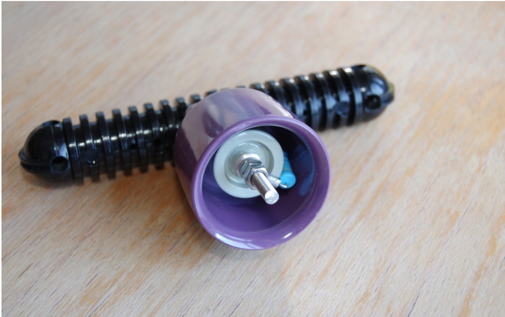
Figure 27: A doorknob capacitor with its snubber resistor installed inside a protective inverted egg cup. The egg cup is made of a durable, weather-resistant plastic. The whole is attached to an antenna insulator.
