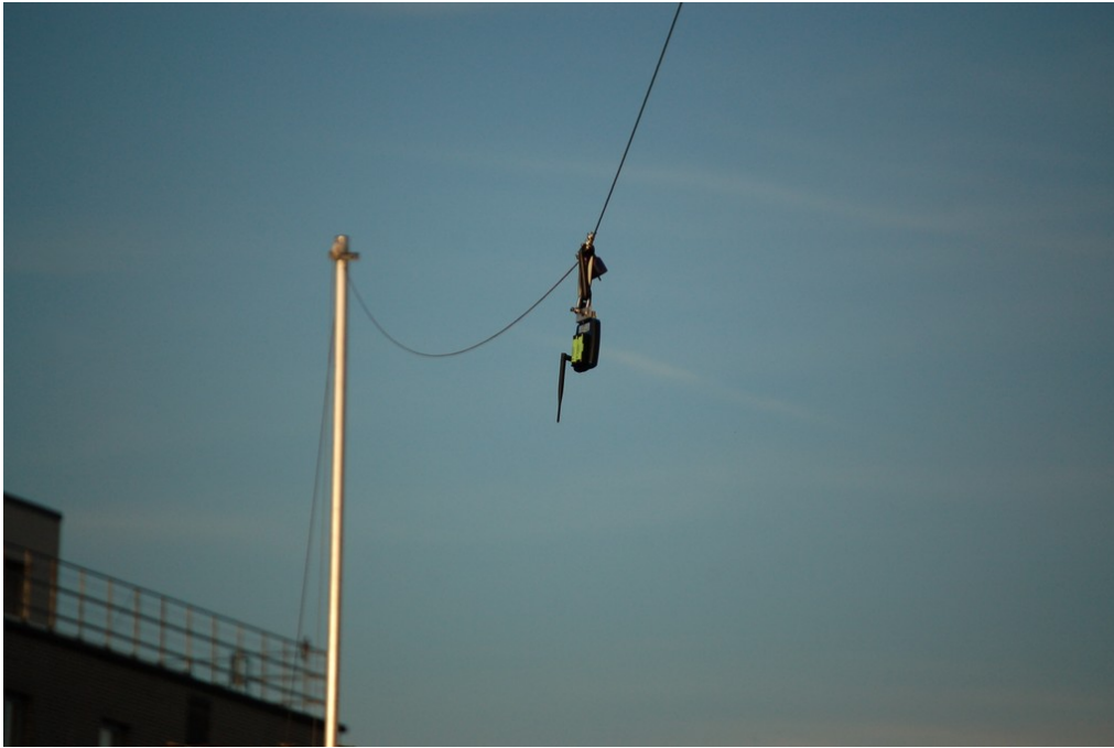
Figure 29: A modified miniVNA PRO hanging from the center of a HF dipole at about 15 m (50 ft) above ground. A balun is not required for taking accurate measurements. The VNA can be read from the comfort of my home even though there are quite some 2,4 GHz WLAN signals present in this urban environment. Two 3350 mAh Panasonic NCR18650B Li-ion cells in parallel provide more than enough «juice» for a whole day of measurements.
