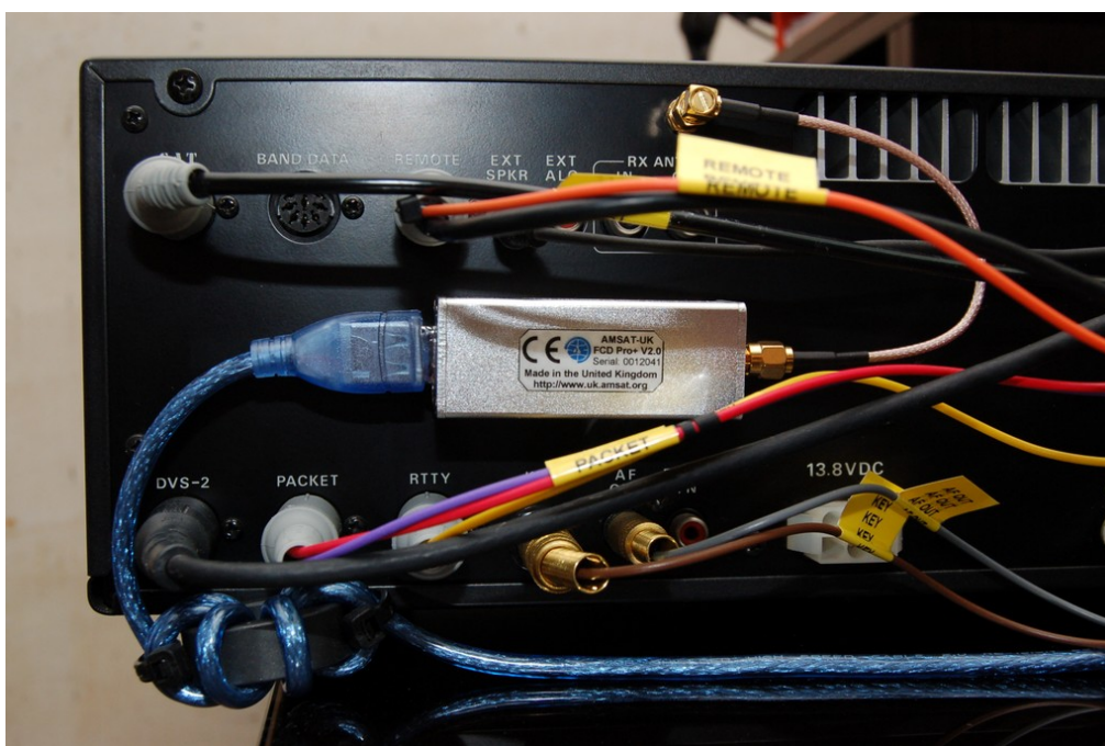
Figure 8: The shielded FUNcube Dongle Pro+ mounted on the modified Yaesu FT-990 with a strip of 3M™ Dual Lock™ hook & loop fastener.
