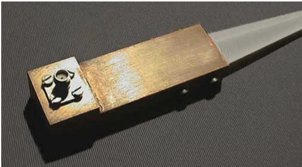
Figure 2: Waveguide feed of the X-band dielectric rod antenna
