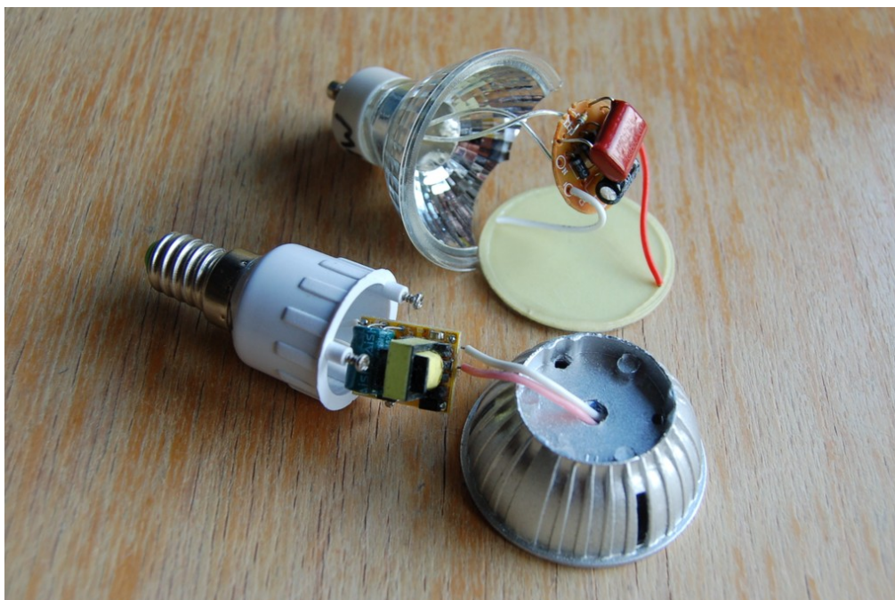
Figure 1: Front: EMI dirty LED bulb with unfiltered buck converter, recognisable by its yellow transformer; Back: EMI clean LED bulb with a big, red-coloured series high-voltage capacitor.
