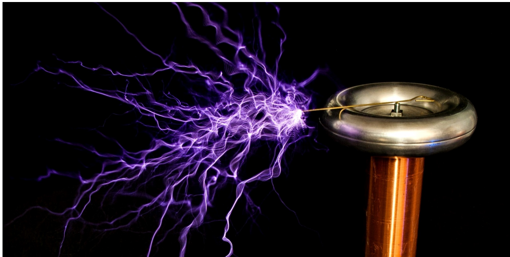
Figure 5: Voltage breakdown of the air at one end of a Tesla coil. Source: oneTesla
