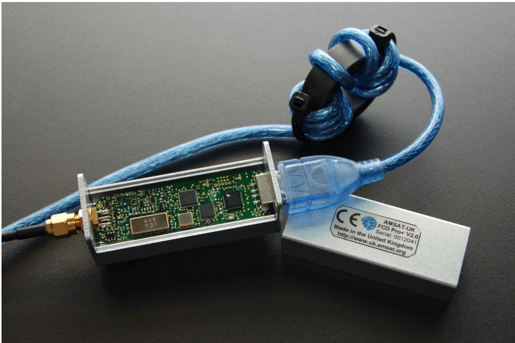
Figure 7: The FCD Pro+ received a new shielded housing. Spinning the USB cable ten times over a FT-140-43 ferrite core results in an effective sheath current choke, keeping PC noise out.
