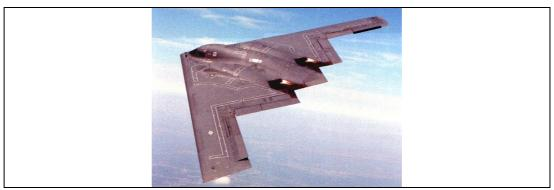
Figure 1.8: The B-2 stealth bomber plane. A flying-wing design and an indented rear edge result in an extremely low RCS value.
