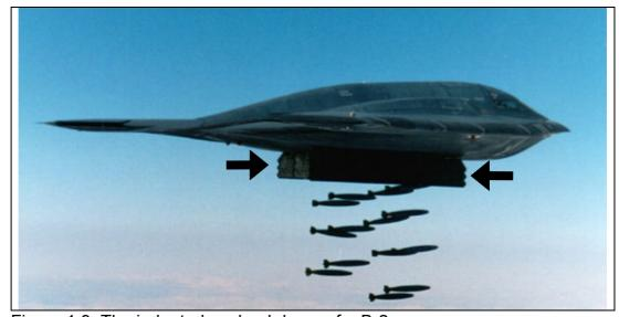
Figure 1.9: The indented payload doors of a B-2
