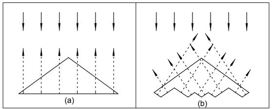
Figure 1.7a: Edge diffraction from the trailing edge of a straight wing Figure 1.7b: Edge diffraction from the trailing edge of an indented wing
