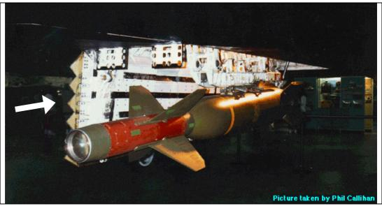
Figure 1.10: A close-up at the indented hatch of one of the F-117A's weapon bays
