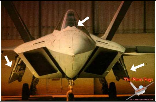
Figure 1.11: Indented surface discontinuities on the F-22's fuselage
