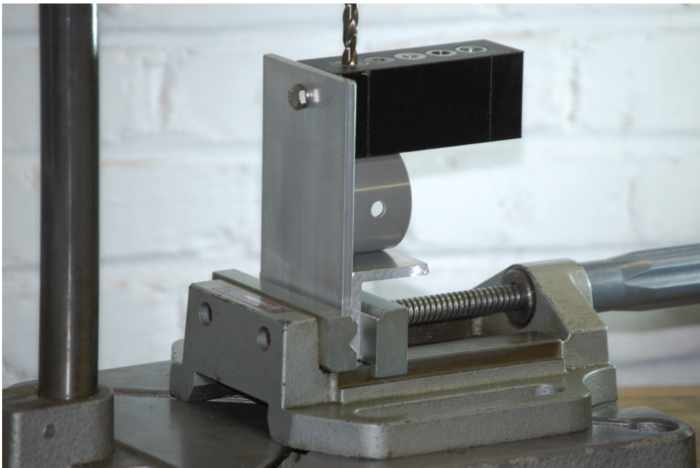
Figure 4: Drilling a PVC spreader for an open star quad line using a slightly modified V-block from Aliexpress. The V-block is screwed against an aluminium back panel. The pipe for the spreader is OD 50 mm thin-walled grey PVC. It fits snugly between the V-block and the pre-drilled aluminium angle stock. The PVC pipe is 36 mm wide, putting the first hole of the V-block at its center. Four holes are drilled two at a time with a \varnothing 7 mm HSS drill bit. Always drill vertically through a V-block and apply ample lubricant to prevent wear of the V-block drill cylinders.
