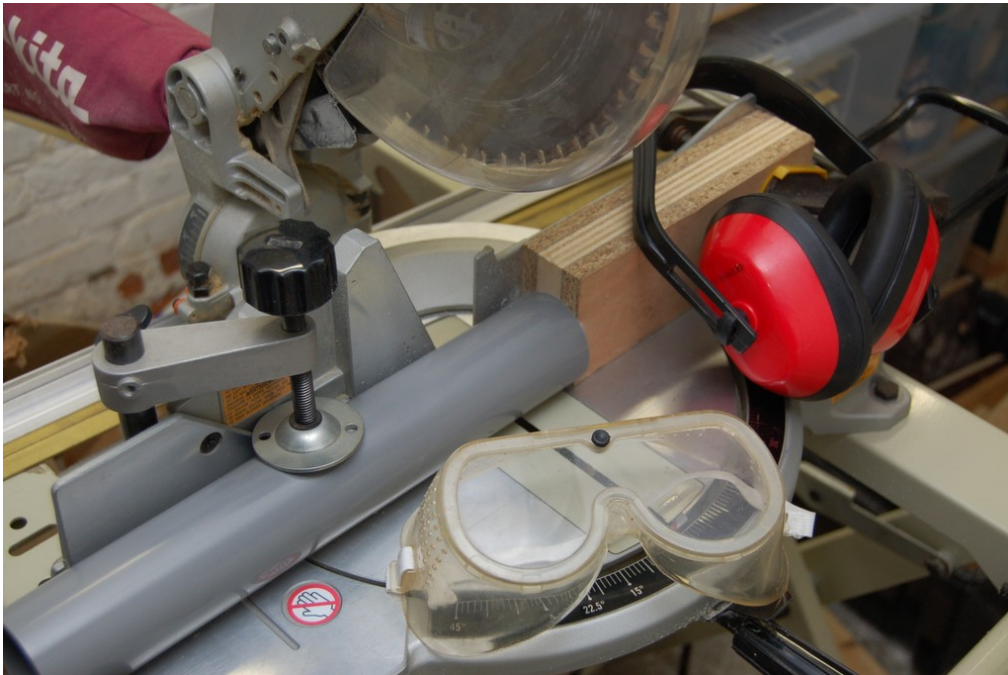
Figure 3: Cutting 36 mm lengths of thin-walled OD 50 mm PVC pipe with a mitre saw. A clamped block of wood at 36 mm from the saw blade serves as an end stop. Use personal protective equipment (PPE) when operating power tools.
